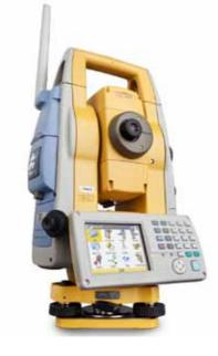
• Scanning, imaging and robotic total station
